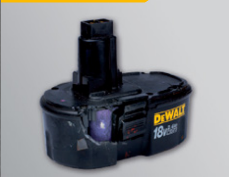
User dropped battery causing severe damage
