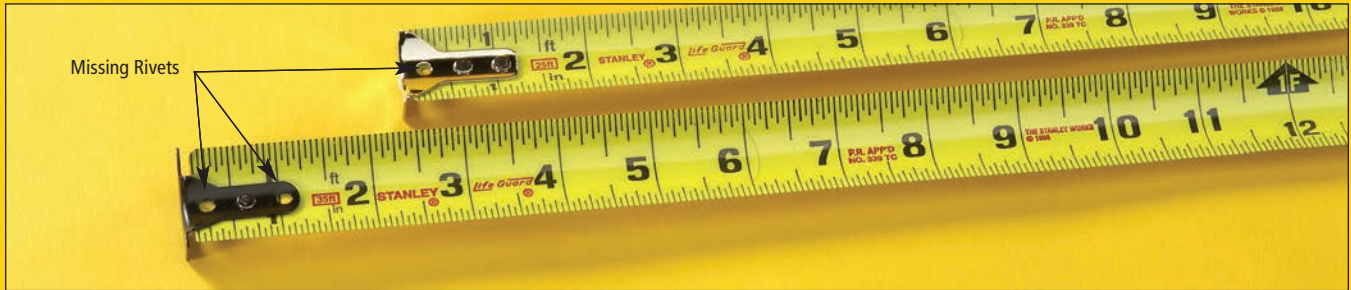
Missing Hook Rivets
